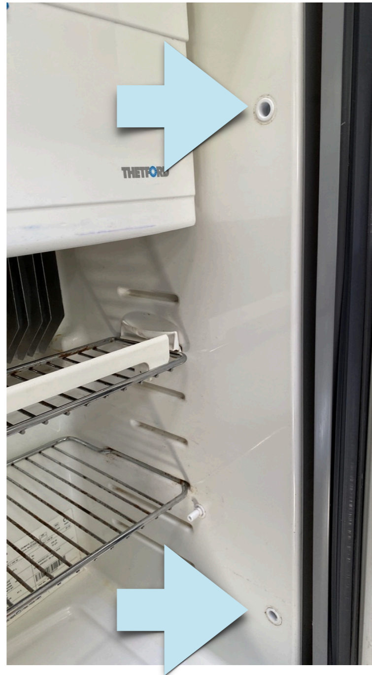
Loosen these 2 screws, there are also 2 on the left.
